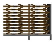
Next panel is placed back-to-back with the first panel by stagger 5 cm. This way the panels rest on the battens and not the foam-strip. Third panel is now placed straight on top, and face-to-face, on the second panel.
