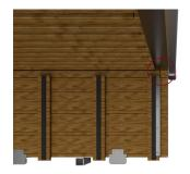
Place the first panel with the face-side down and move to the corner of the end-bar in one of the sides (marked with red circle).
